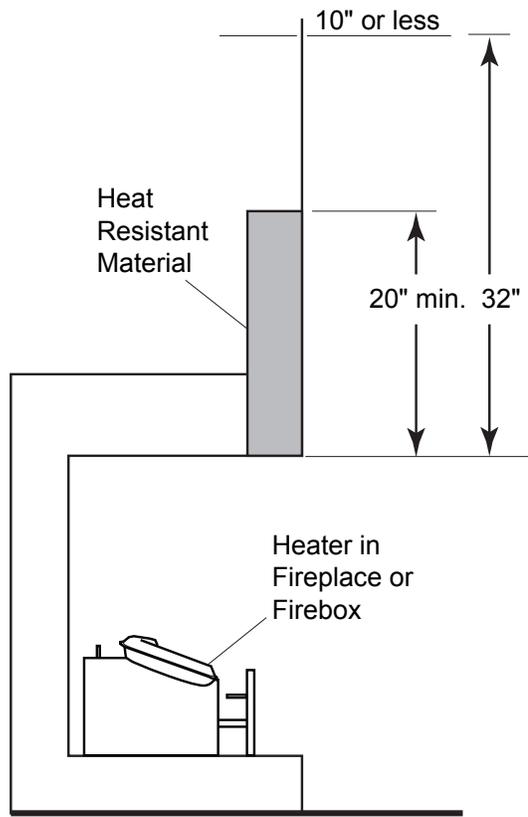
**Figure 8 - Minimum Mantel Clearance with No Hood**
