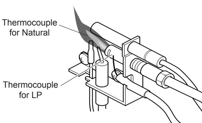
Figure 19 - Correct Appearance of Pilot Flame
