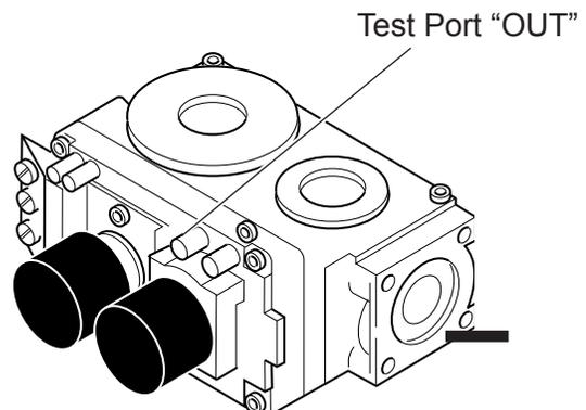
**Figure 15 - Pressure Test Point Location
