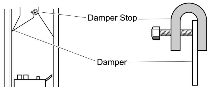
**Figure 11 - Damper Stop Installation.**
