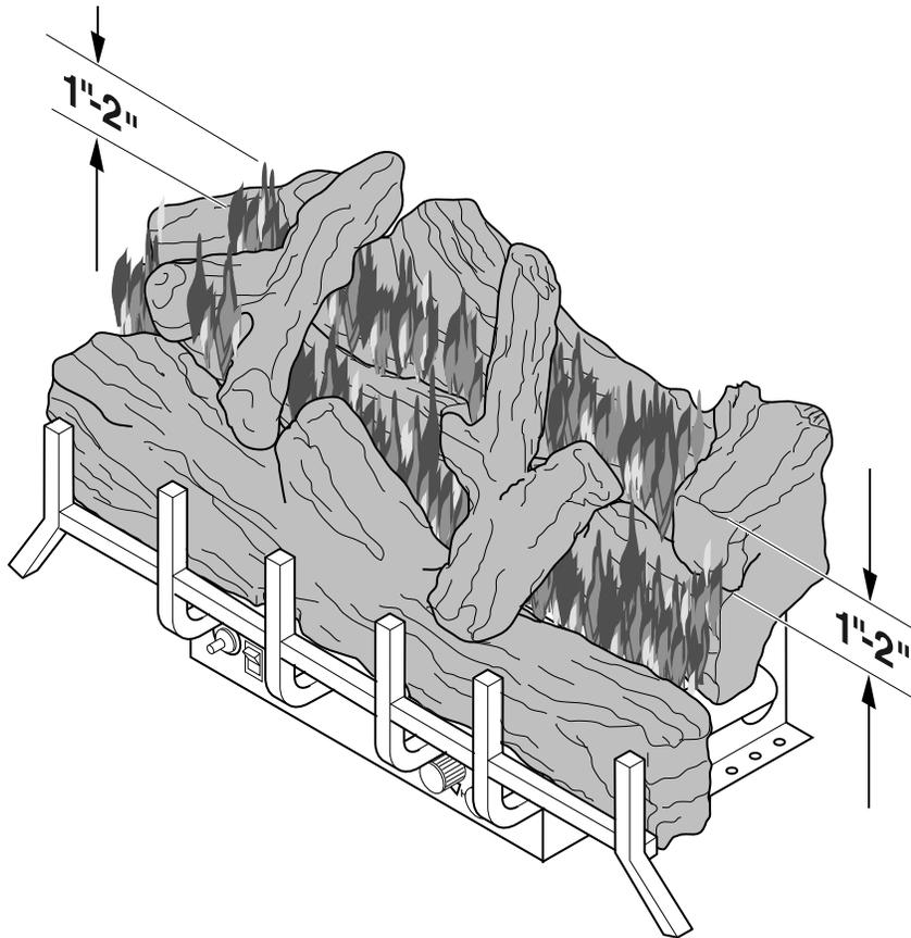
**Figure 23 - Correct Appearance of Rear Flames**
