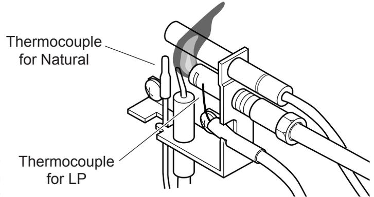
**Figure 20 - Incorrect Appearance of Pilot Flame**
