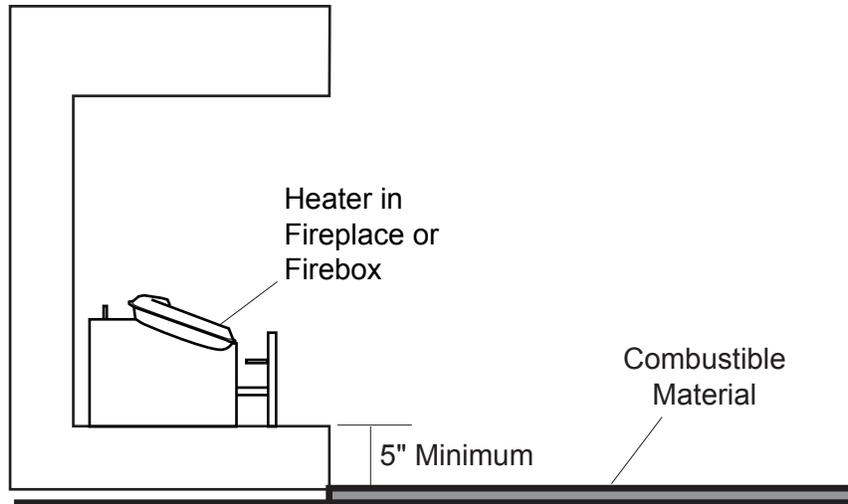
**Figure 9 - Minimum Clearance above Combustible Flooring**
