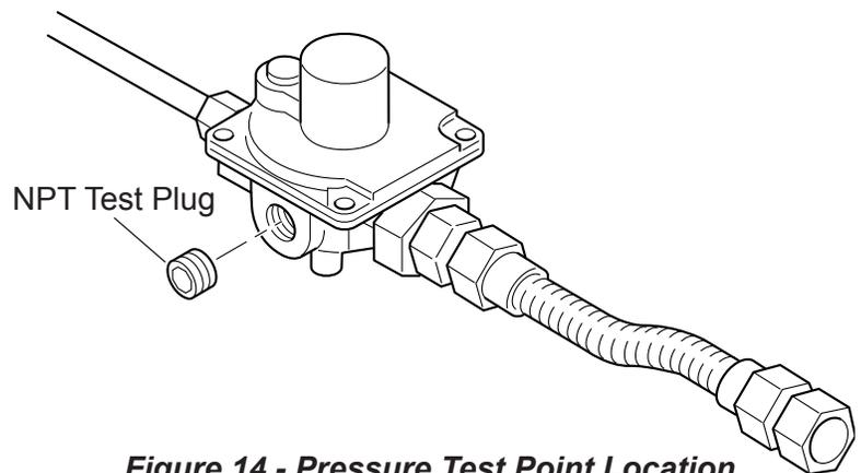
**Figure 14 - Pressure Test Point Location
