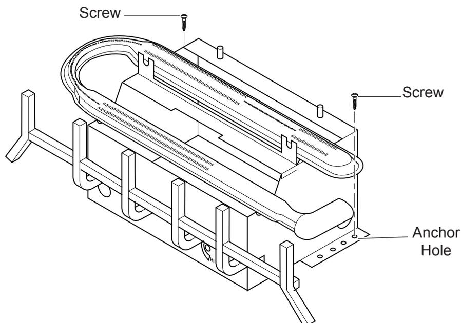
**Figure 12 - Securing Heater to Floor of Fireplace/Firebox**
