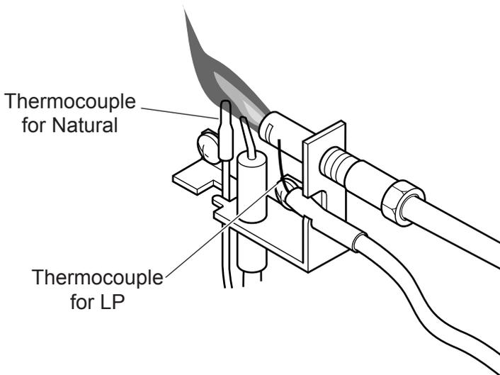
**Figure 21 - Correct Appearance of Pilot Flame**
