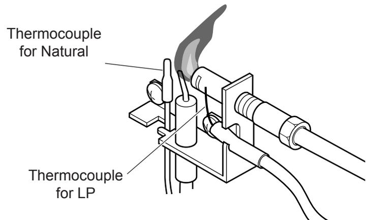
**Figure 22 - Incorrect Appearance of Pilot Flame**
