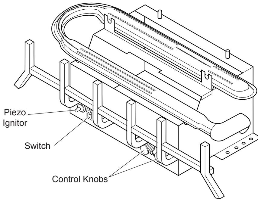
**Figure 24 - Location of Piezo Ignitor, Control Knobs and Switch on Millivolt Unit**
